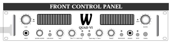
INPUT Socket for the connection of a bassGAIN Control + LED to adjust the input level.LED lights greenMinimum signalLED lights yellowTube compression
