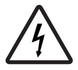
This symbol, wherever it appears, alerts you to the presence of uninsulated dangerous voltage inside the enclosure--voltage that may be sufficient to constitute risk of shock.
